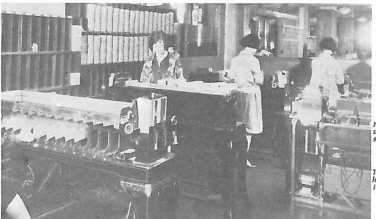
Hollerith punch-card equipment as used in 1931 to mechanize and simplify paperwork.
